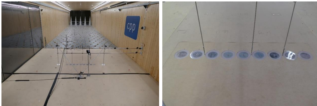
Figure 2. Sensors within the boundary layer wind tunnel including three hotfilm reference sensors.
